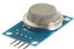
Fig-10: GAS SENSOR
